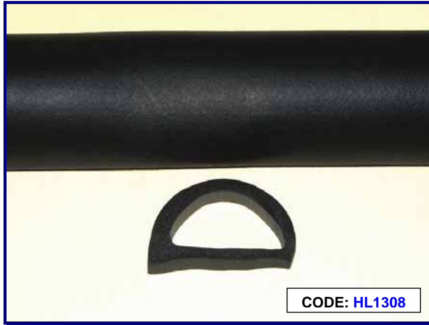
Gasket, 'D' Shaped Sponge High/Low, Polyplas Available: 30mm Wide x 16mm High with 3mm to 4 mm Wall in 50 mtr Roll
