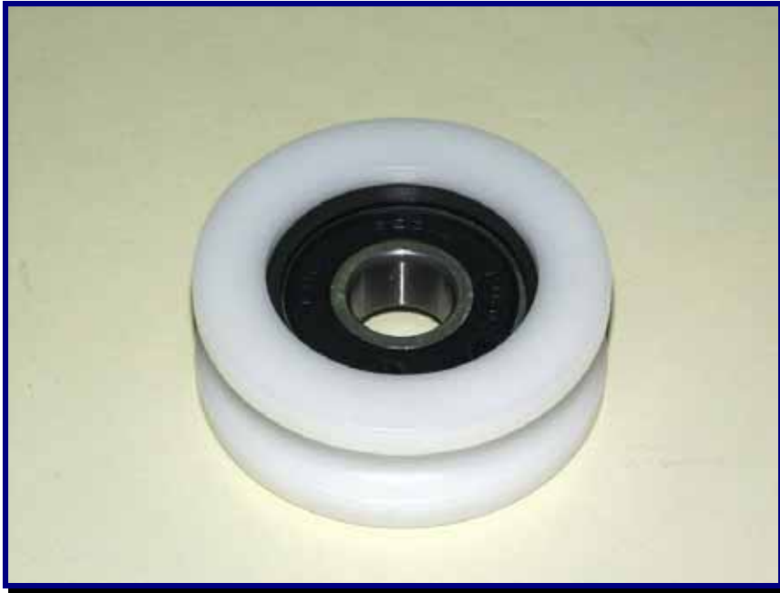
Wheel 'U' Profile, Bearing 12mm ID, Black Steel Circlip, Polyplas / Delrin 50mm OD Suit: Commercial Hanging Roller Assembly
